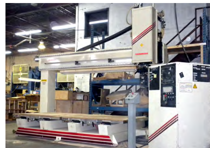
Thermwood 67 with 5-Axis CNC contour router
