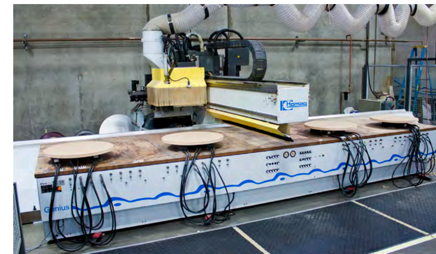
4-Axis CNC router with 3mm universal edge bander
