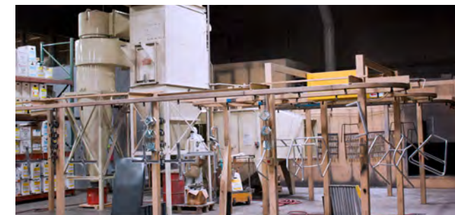
In-house Conveyorized Powder Coat application center
